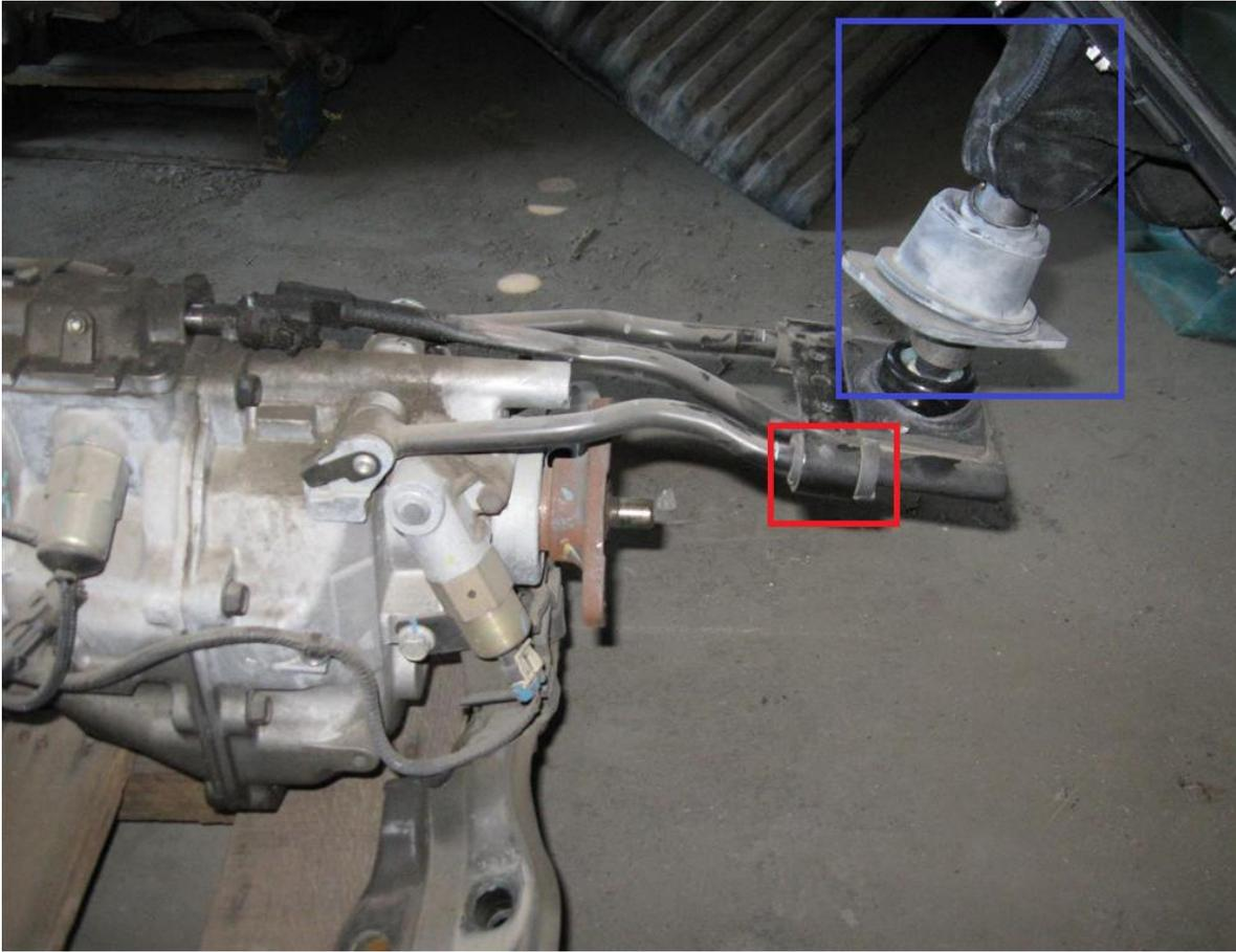
Putting your Creative Steel shifter in the car may now require two people. It is possible to put the shifter onto the linkage base plate (with the zerk fitting towards the rear) with the bolts through the holes, and then crawl under the car and tighten them with two wrenches. Note that the washer goes under the nut, not under the head of the bolt.
