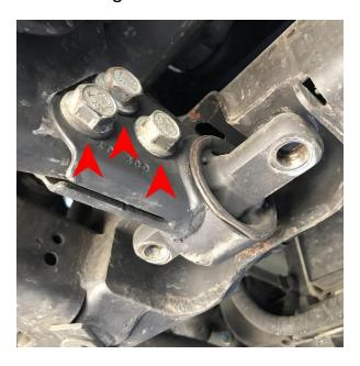
5. Put both 12" extensions and 18mm socket on one ratchet and 6" extension and 15mm socket on the other ratchet. Remove the nut from the bolt going through the
