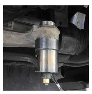
10. Now set the tool up the same way on the pinion bushing and remove the bushing. Make sure the notch in the cup is lined up with the differential housing.
