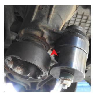
11. After removing both OEM bushings, make sure that the bore on both pinion and passenger bushing housings are clean and free of any burrs. Both OEM bushings need to be removed entirely like shown.
