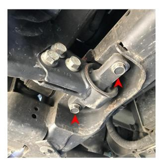
4. Using 3/8" drive ratchet and 18mm socket as well as the 18mm wrench, remove the three bolts that hold the front bushing to the differential.
