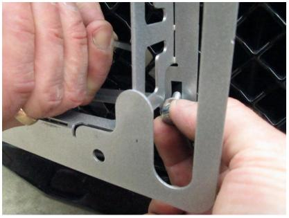
6. Tighten the bolts with a 7/16" wrench and cut off zip tie.
