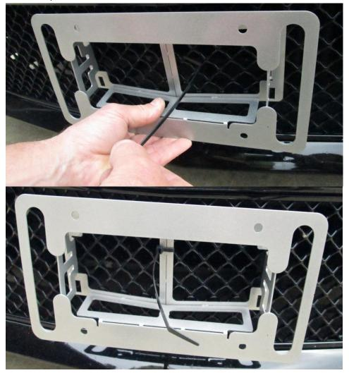
5. Use the small tab on the sheet metal nuts as a handle while installing the bolts. Ensure the washers are placed between the bolt and the license plate bracket.
