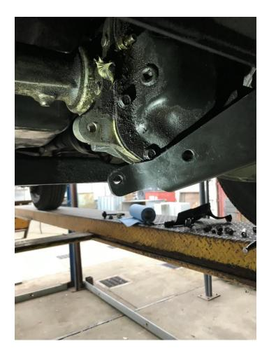
5. Remove plastic oil drain catch using 10mm socket. (it is a pain to remove but it will come out.
