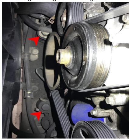
4. Using 13mm socket remove the 3 bolts that hold the front differential mount to the differential. Move mount to the side like shown.
