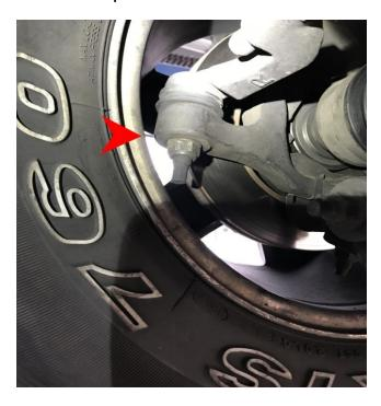
7. Now that everything is loose you can move the steering rack into this position to remove the bushings.
