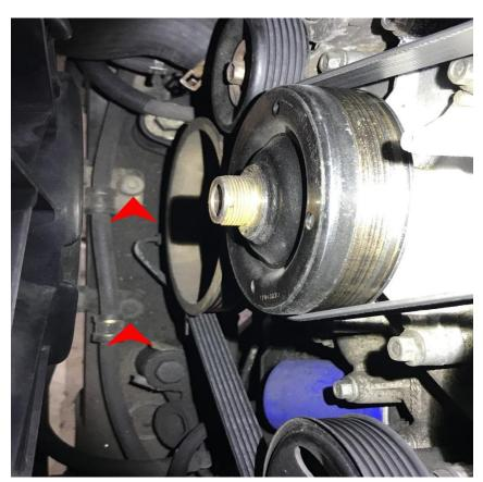
2. Using a 13mm socket and 12" extension remove the steering linkage bolt. (fist picture shows bolt that needs to be removed and second picture shows how to gain access to bolt. You may need to turn the steering wheel for proper lineup with socket)
