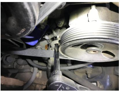
3. Using 24mm socket on bottom and 24mm wrench up top, remove the 2 large steering rack mounting bolts.
