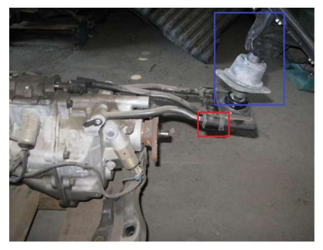
Putting your Creative Steel shifter in the car may now require two people. It is possible to put the shifter onto the linkage base plate with the bolts through the holes, and reach around the base plate or crawl under the car and tighten the nuts with a 13mm wrench/socket. Don't over tighten, torque spec is only 15-20ft/lbs. After tightened up, you can reinstall the rubber boot, putting the wide sections over the head of the bolts.
