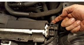
Next remove the supercharger belt by using a 12 point 17mm wrench on the belt tensioner.
