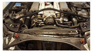
Next you will need to remove the fiberglass panels under the engine compartment. Using a 8mm socket, remove the four screws from the first panel and six screws from the second.
