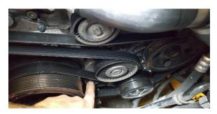
Remove the double idler by prying off the plastic cap and using a T50 torx to remove the bolt.
