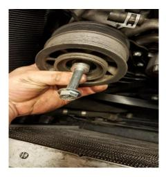
Using E10 socket, remove water neck bolt.
