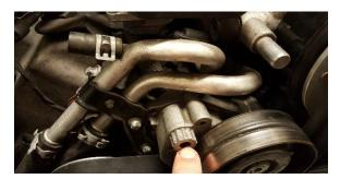
Remove the accessory belt using a 17mm socket on the belt tensioner.
