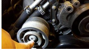
Reinstall double idler using 10x100mm bolt and spacer with Loctite. Leave bolt loose enough for BWK front plate.
