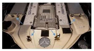
Remove Core support sheet metal using 10mm socket and T30 torx. There are three bolts on each side and three bolts in the center. Lastly remove the plastic pins by prying up on them.
