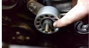
Reinstall accessory belt. Install new supercharger belt. Install BWK front plate with 10mm nut using Loctite and 15mm socket. Ensure to tighten double idler bolt using 15mm socket. Install everything else in reverse order of removal. Any questions feel free to call us at (503) 316-1811.
