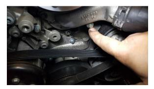
Using 15mm and 8mm sockets, install BWK rear plate like shown. Ensure to use Loctite on both bolts and careful not to tighten the small bolt too much as the aluminum is soft and can strip. Ensure washer is on stud in front of nut.
